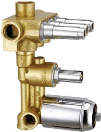
ALD-4004B 40 mm High flow diverter body with 2 inlets & 4 outlets Push Button Type
